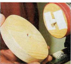
03 Push the turned disc on a home-made glue chuck with a dowel centre pin. Carpet tape will hold the work for drilling
