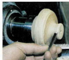
02 Use a firm parting tool to roll the beads and cut the fillets, taking light cuts and keeping the detail sharp
