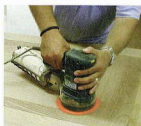
15 Sand the assembled doors. I used a random orbit sander to reduce the amount of swirls formed on the surface
