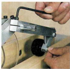
Hold-down wheels are mounted on aluminium bars and locked tight with hex grub screws. The bars can be raised on the rear vertical rod
