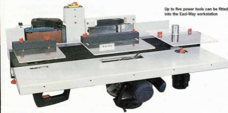
You need to fit the circular saw so its guard stays retracted below the table
