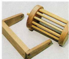
10 The frame and the handle ready for assembly. Make sure the balls are inside before gluing the final piece of dowel
