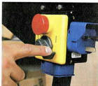
The NVR switch has a 13A plug at the side and a router socket underneath
