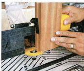
Plastic hold-downs fit into slots on the table or on the fence itself
