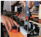
You can adjust the squareness of the fence with a couple of screws
