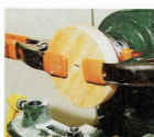
04 Cramp up the wood to the chuck with its carpet tape for a few minutes to improve adhesion
