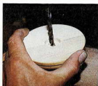
06 Use a 9mm drill to a depth of 8mm. This is deep enough to accommodate the screw head
