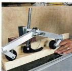
This is arguably the 'best hold-down system of the lot. Wheels are canted so that the workpiece feeds in towards both fence and table
