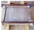
14 Glue up the door frame, but don't apply glue to the panel edges. Measure the diagonals to check for square
