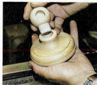
12 Gluing should be no problem as long as they're a good fit. Put a little glue on the spigot and push it into place
