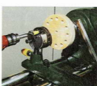
05 Drill 12 holes using a drilling jig. The tape on the drill acts as a depth stop. A small cordless drill is useful for this
