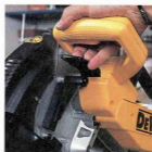
A paddle lever releases the lock on the guard in order to drop the head
