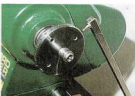
The faceplate has 24 holes for indexing. The lathe is locked in place with the indexing arm and its pin
