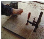
15 Round over the edges of the top panel with a router. The top is fixed by screwing up through the top rails
