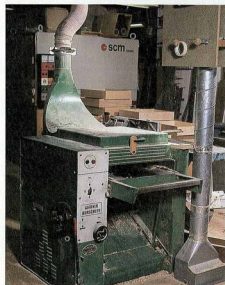
The Wadkin thicknesser, 30 years old and still in daily use, sits alongside many more modern pieces of kit
