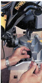
Each side of the fence can be moved sideways to enable the head to tilt
