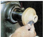
04 After sanding and sealing, rub back with 0000 wire wool in preparation for your final finish
