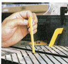
Plastic hold-downs fit into slots on the table or on the fence itself
