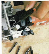
Each dowel bit is locked in place with a hex grub screw. A wrench is supplied
