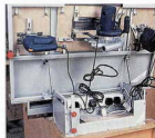
The table is hinged for access. Power tools all plug into a mains board
