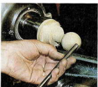
09 Remove the tailstock and use a 6mm gouge to finish turning the end of the ball. Include a decorative button on the end
