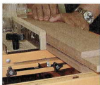
10 Form the grooves in the matchboard rails and stiles at the same setting as before. There are no rebates at all
