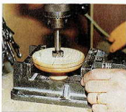
05 With a 25mm Forstner bit, drill to 5mm. This will leave the brass plate and the screw heads below the surface
