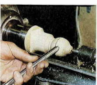
08 Fix the blank on to the screwchuck and put a pencil mark around the centre to give an indication where the hole is
