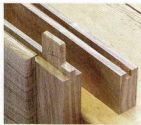
13 A groove is run around the edge of the panel to enable it to fit inside the rails. The exposed edge is rounded over
