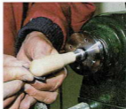
09 The handle is held firmly on the stepped friction drive and the tailstock moved away for final sanding
