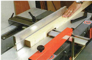
An aluminium bridge guard is fitted, while the planer fence can be tilted to about 30°. The saw's sliding carriage can be tilted to 45°, but bevel cutting is tricky
