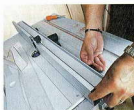
You can slide both sides of the fence outward to suit the cutter diameter. The fence is box section aluminium
