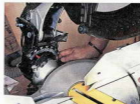
The protractor scale for bevel cuts is easy to read and can be calibrated
