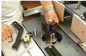
Standard equipment includes a CMT cutterblock. This is fitted with 40mm HSS straight knives. A huge range of cutters is available for moulding profiles
