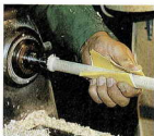
11 Sand the dowel, first with the lathe running. Stop the lathe and rub up and down to eliminate any sanding marks
