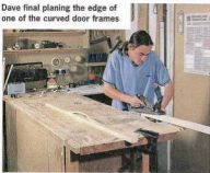
Dave final planing the edge of one of the curved door frames
